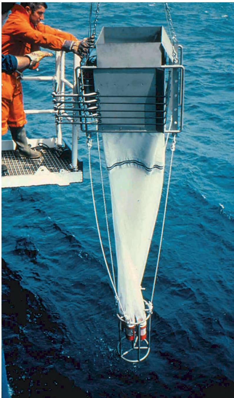
*The Multinet consists of five or more nets which can be opened and closed sequentially to sample subsequent depth layers while the gear is vertically hauled. Photo:W Hagen*
